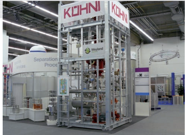
At Achema 2009, Kühni presented the plant designed for Weyland A/S and joined together as skid for acid recovery.
